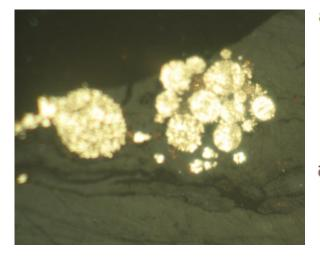
Fig 5. Pyrite framboidal associated with desmocolinite in coal, reflectant white light, 500x. Sample 6105/16.
