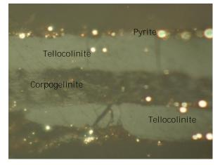
Fig 4. Corpogelinite and pyrite associated with desmocolinite in coal, reflectant white light, 500x. Sample 6103/16.
