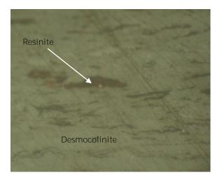
Fig 3. Resinite associated with desmocolinite in coal, reflectant white light, 500x. Sample 6105/16.
