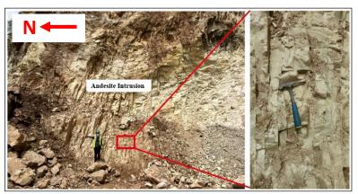
Fig 3. Weathered hypersthene-andesite in Bobos quarry
