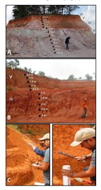
Fig.7 Field observation activities. (A, B, C) outcrop descriptions, thickness measurements in each weathering zone, undisturbed sampling.
