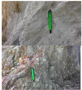
Fig 5. Fault breccias and slicken side feature indicating the slope was affected by a fault system.
