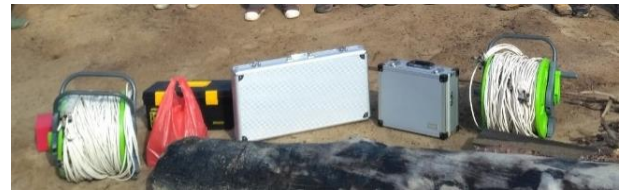
Figure 3. Equipment of Vertical Electrical Sounding (VES)
