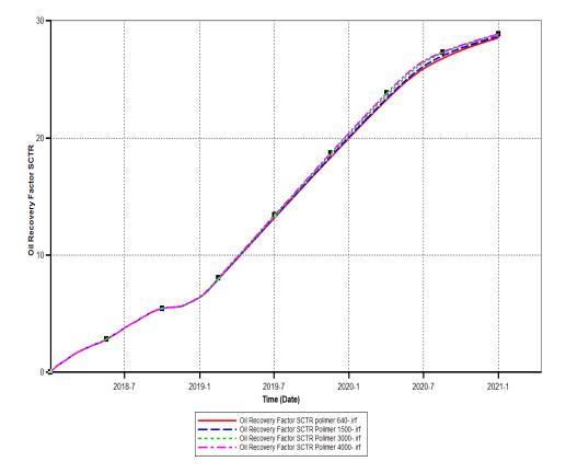
Fig 1. Effect of polymer concentration on oil recovery factor
