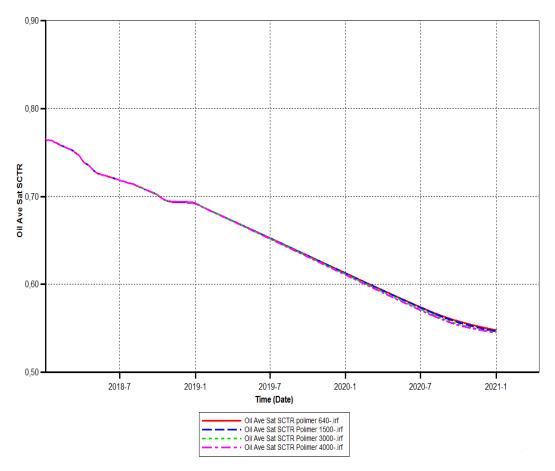
Fig. 2. SOR reduction after polymer flooding by various concentrations
