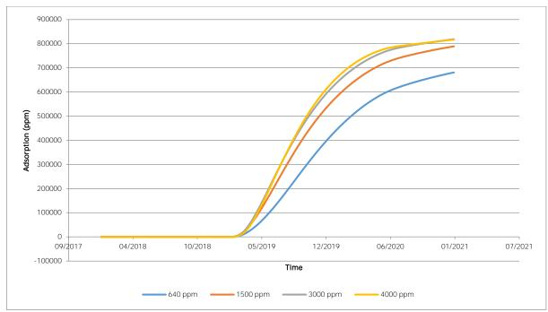
Fig. 3. Polymer adsorption at various polymer concentrations
