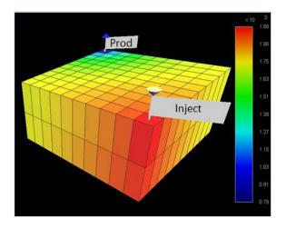
Fig. 4. Pressure final condition after polymer flooding
