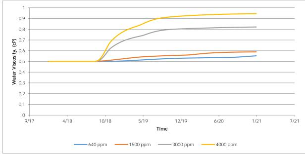
Fig. 7. Increasing water viscosity by various concentrations of polymer flooding.
