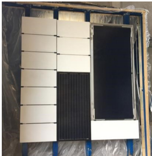
FIG. 11 Performance mock-up of the façade integration, passive (left), PV (centre), and ST (right) claddings
