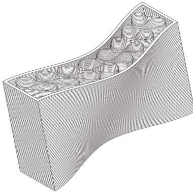
FIG. 8 S-Brick extrusion path model.
