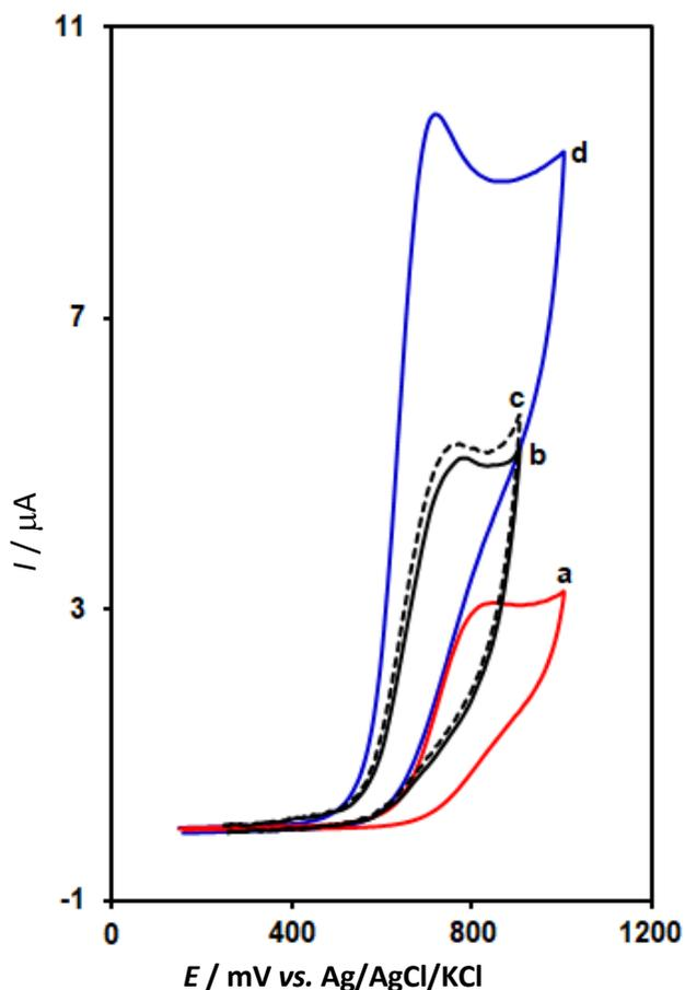
**Fig. 3.** CVs of a)  $\text{Fe}_3\text{O}_4@\text{SiO}_2/\text{GO}/\text{SPE}$  and b) unmodified SPE in the presence of  $100.0 \mu\text{M}$  tryptophan at pH 7.0. In all cases, the scan rate was  $50 \text{ mV s}^{-1}$
