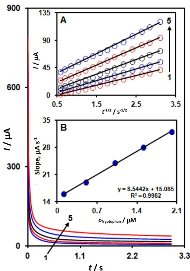
**Fig. 5.** Chronoamperograms obtained at  $\text{Fe}_3\text{O}_4@/\text{SiO}_2/\text{GO}/\text{SPE}$  in 0.1 M PBS (pH 7.0) for different concentrations of tryptophan. The numbers 1–5 correspond to 0.1, 0.5, 1.0, 1.5 and 2.0 mM of tryptophan. Insets: (A) Plots of  $I$  vs.  $t^{-1/2}$  obtained from chronoamperograms 1–5. (B) Plot of the slope of the straight lines against tryptophan concentrations.
