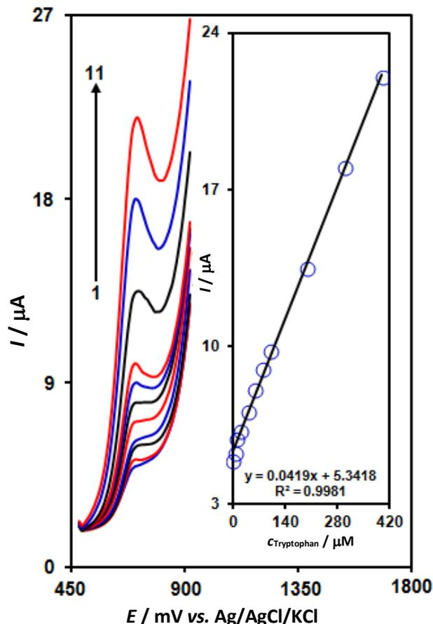
**Fig. 6.** DPVs of  $\text{Fe}_3\text{O}_4@/\text{SiO}_2/\text{GO}/\text{SPE}$  in 0.1 M PBS (pH 7.0) containing different concentrations of tryptophan. Numbers 1–11 correspond to 1.0, 5.0, 10.0, 20.0, 40.0, 60.0, 80.0, 100.0, 200.0, 300.0 and 400.0  $\mu\text{M}$  of tryptophan. The inset shows the plot of the peak current as a function of the tryptophan concentration in the range of 1.0–400.0  $\mu\text{M}$ .
