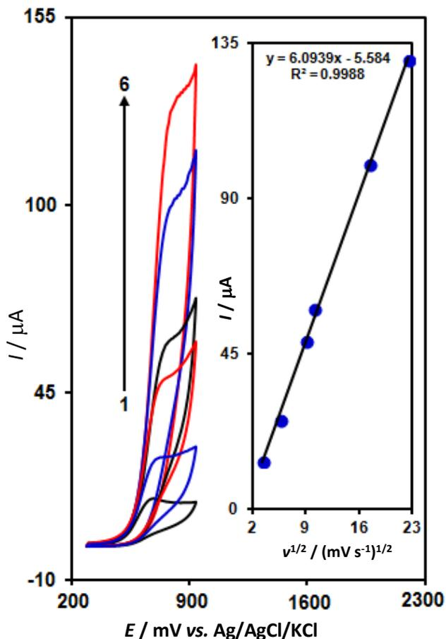
**Fig. 4.** CVs of  $\text{Fe}_3\text{O}_4@\text{SiO}_2/\text{GO}/\text{SPE}$  in  $0.1 \text{ M}$  PBS (pH 7.0) containing  $200.0 \mu\text{M}$  of tryptophan at various scan rates; numbers 1–6 correspond to 10, 30, 80, 100, 300 and  $500 \text{ mV s}^{-1}$ , respectively. Inset: Variation of anodic peak current vs. square root of scan rate
