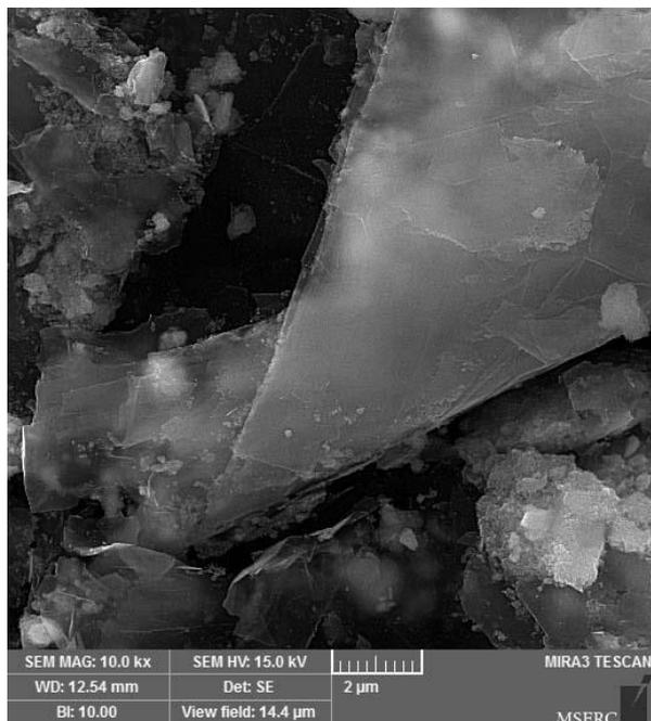
**Fig. 1.** SEM image of Fe<sub>3</sub>O<sub>4</sub>@SiO<sub>2</sub>/GO nanocomposite
