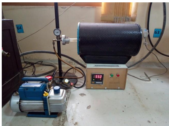
Figure 1. Vacuumed furnace system
