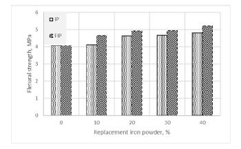
Figure 7 Effect of waste iron powder on flexural strength at different age.
