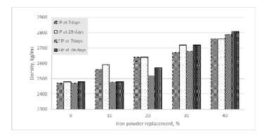
Figure 1 Effect of waste iron powder on hardended density at different age
