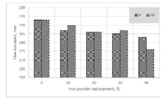
Figure 4 Effect of IP and FIP replacement on flowability cement mortar
