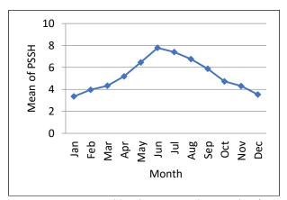
Figure 3 Average monthly solar energy on horizontal surface
