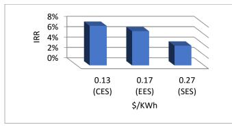
Figure 11 Relationship between IRR and Energy system cost
