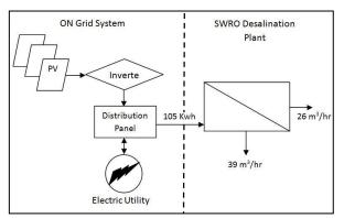
Figure 9 SWRO Plant depends on On Grid System
