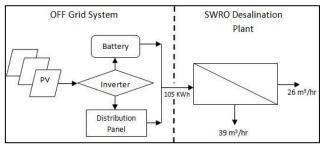
Figure 8 SWRO Plant depends on Off Grid System
