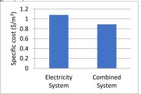
Figure 14 Specific Cost of Desalinated Water
