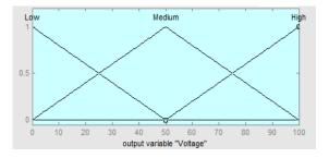
Figure 7 Output membership function plot for voltage
