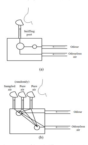
Figure 1: Types of dynamic Olfactometer (a) Yes/No method (b) Force-choice method
