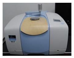
Figure 6 Fourier Transform Infra-Red (FTIR)
