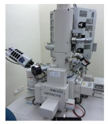
Figure 3 Field Emission Scanning Electron Microscopy (FESEM)
