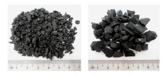
Figure 1 Waste tyre rubber (Rubber Granules)
