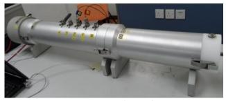
Figure 7 Impedance Tube
