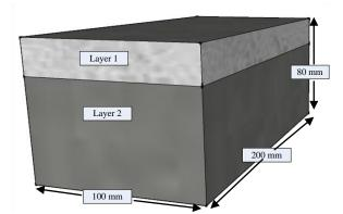
Figure 2 Double Layer Rubberized Concrete Paving Block (DL-RCPBs)
