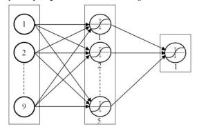
Figure 4: The architecture of the MLP model.
