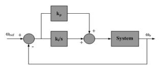
Fig. 9- Block Diagram of a PI Controller
