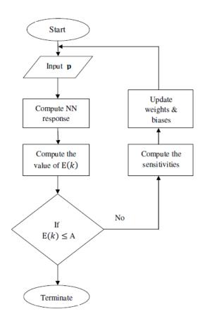
Figure 3: Flow chart of the steepest descent algorithm
