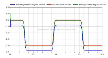
Figure 4: Simulation of computed torque control in the presence of structured uncertainties
