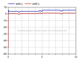
Figure 9: Sum of the outputs of PD and FFC controllers after adding the NOTC
