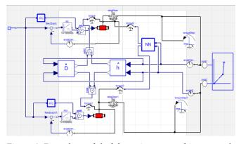
Figure 2: Dymola model of the trajectory tracking control system
