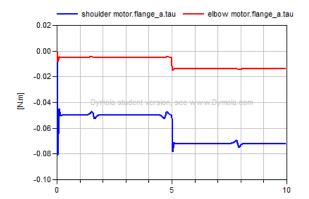
Figure 7: Disturance torques on the motors before adding the NOTC
