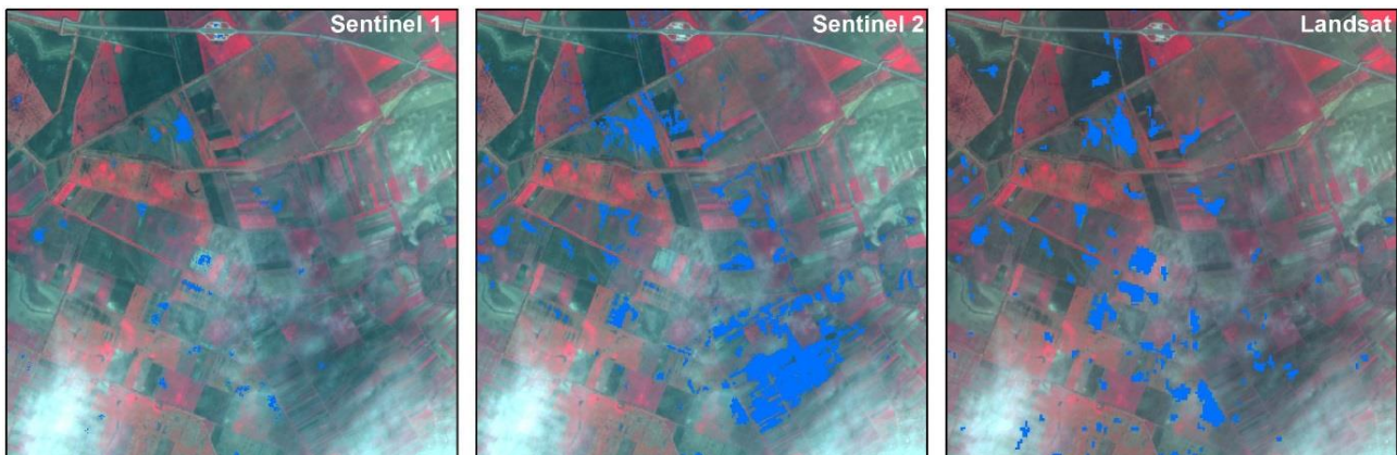
Fig. 5 Sentinel 2 false colour composite (RGB 843) covered with the results of the three separate processing workflows
