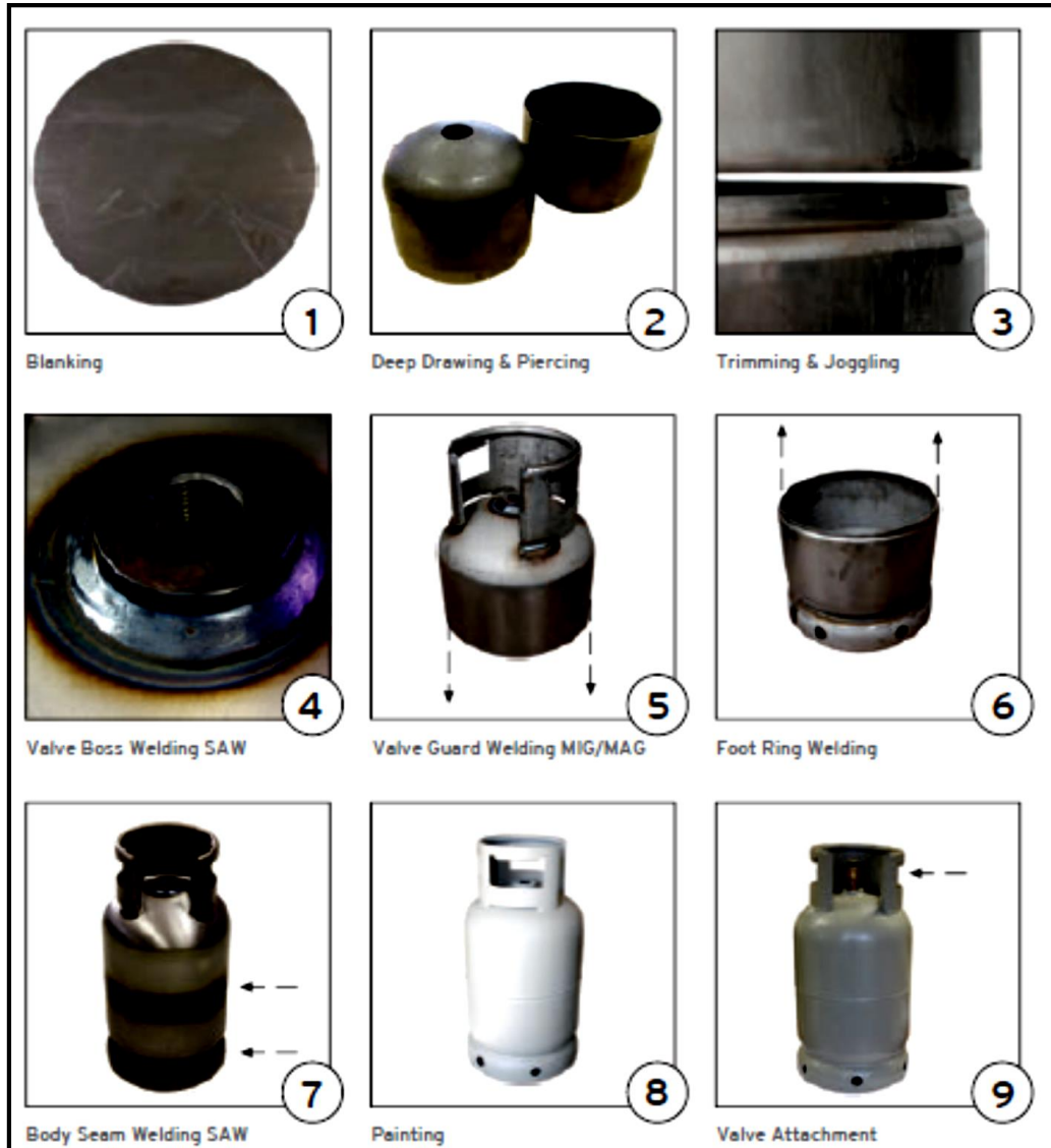
Figure 1. The processes of manufacturing LPG cylinders [5]
