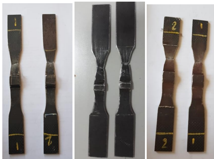
Figure 4. Tensile test samples (weld metal)
