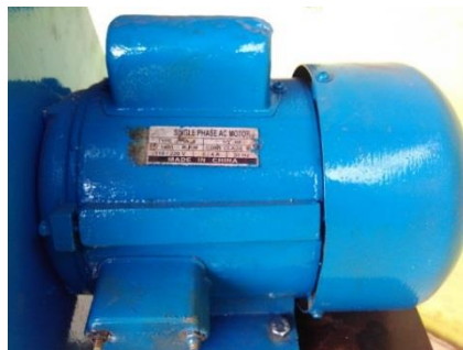
Figure 6. Dynamo ADK Electric Motor Type JYIA-4 1 phase 0.50 HP
