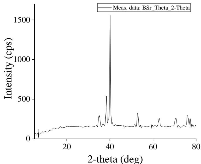
Figure 8. XRD results at HAZ and Fusion Zone
