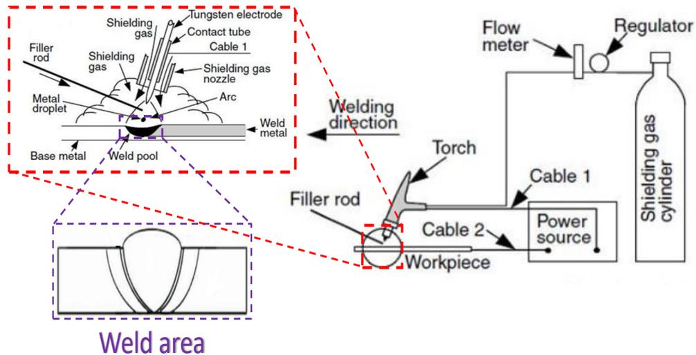
Figure 1. Schematic of the GTAW equipment used
