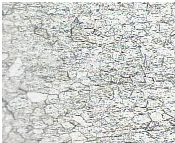
Figure 6. Parent metal microstructure
