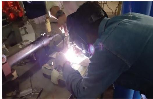
*Figure 2. GTAW welding process on titanium*
