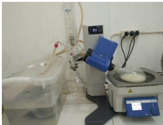
Figure 4. Corncob fermented distillation
