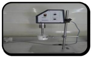
Figure (1): Ultrasonic Probe
