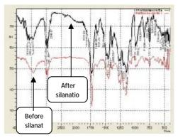
Figure (4): Polymer Nano Composite before and after Silanation
