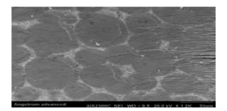
Figure (6): SEM of PMMA/Zrsio4 Nanofiller
