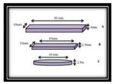
Figure 1: Test specimens A: Impact test, B: Transverse test, C: Thermal conductivity test.
