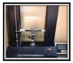
Figure 5: Instron testing machine.
