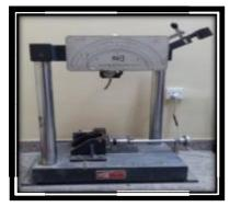
Figure 3: Impact testing devise (charpy type)
