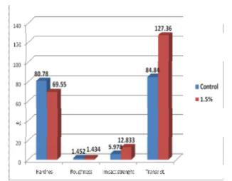
Figure 1: Bar chart of the mean values for hardness, roughness, impact strength and transverse strength for both control group and 1.5 % SWCNTS
