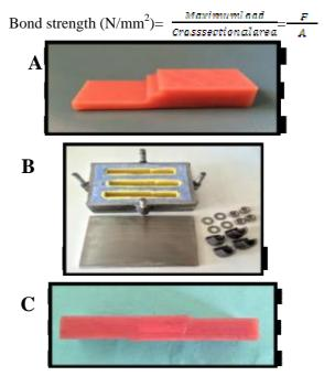
Figure 2: (A) Acrylic block used in test, (B) Custom-fabricated flask with silicon-stone mould. (C) Shear bond strength test specimen.
