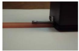
Figure 3: Profilometer (portable roughness tester)
