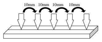
Figure 2: Schematic diagram of the surface hardness test specimen with five test sites.
