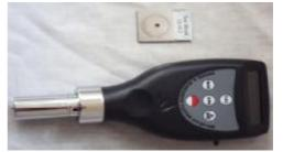
Figure 1: Compact portable indenter (Shore D hardness tester) with its test block.
