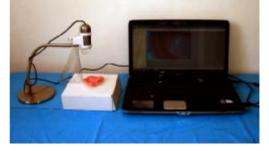
Fig. 3: Measurement of linear dimensional changes using digital microscope
