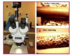
Figure 1-a.stereomicroscope, (b, c implants as appearing under stereomicroscope) b .cylindrical compacted implant before sintering, c. cylindrical compacted after sintering
