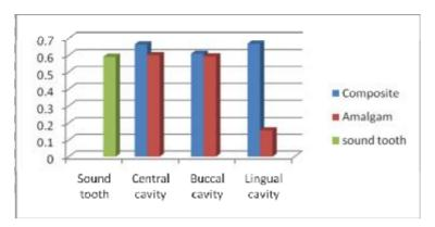
Figure 3: Displacement vector sum in mm according to cavity position and filling materials used.
