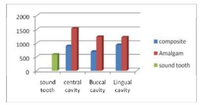
Figure 2: Maixmum Von Mises stress recorded according to the model in MPa
