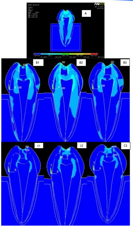
Figure 4: Stress pattern of the maximum Von Mises stresses according to the model. A sound tooth structure, B1,B2, and B3 are of composite restoration in central, buccal and lingual cavity position respectively. C1, C2, and C3, are of amalgam restoration in central, buccal and lingual cavity position respectively.
