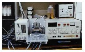
Figure 4: Flameless atomic absorption spectrophotometer.
