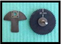
Fig. 10: Horizontal plate insertion guide and disk drill
