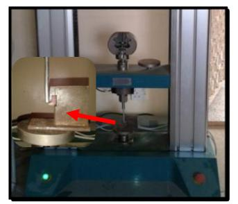
Figure 3: Instron machine with tooth clamp
