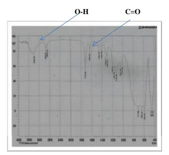
Figure 4b: FTIR of treated PP fibers with (C=O, 1719) and (O-H, 3382) functional groups.
