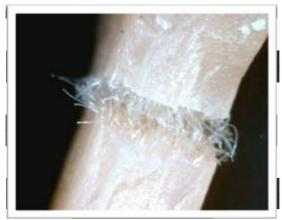
Figure 6: Tensile strength PP fiber reinforced specimen after submitting to the test.
