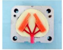
Fig. 1: Wax sprues attached to wax patternsin vertex thermo flask
