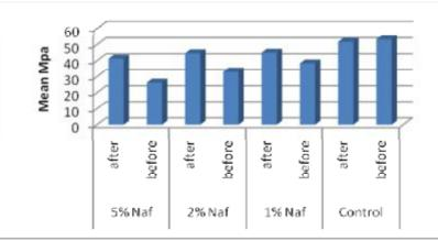
Figure 2: The mean value of tensile strength test
