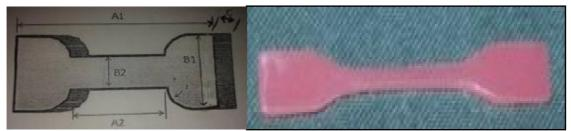
Figure 1: Dimensions of the specimens of tensile strength test
