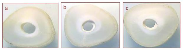
Figure 3: Different failure modes. (a) Adhesive failure; note clean canal wall. (b) Cohesive failure; within tested material. (c) Mixed failure; note the material residual inside the canal.
