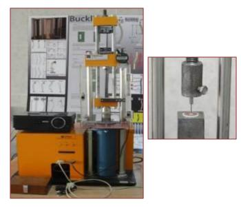
Figure 2: Digital universal testing machine with the tested sample.
