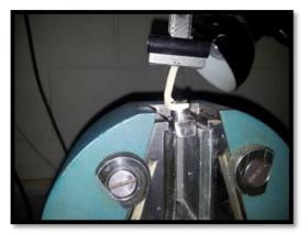
Figure 4: Testing procedure of Acetal and co-cr clasps,
