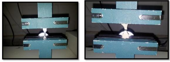
Figure 5: Testing procedure of Acetal and Co-Cr tensile samples.
