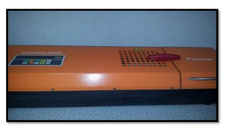
Figure 3: Acetal flexite injection machine.
