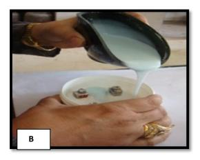
Figure 2: Wax models after casting by crown and bridge metal. B. Duplication of the metal models by poly vinyl siloxane duplicating material.
