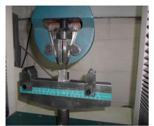
**Figure 6: Universal testing machine**
