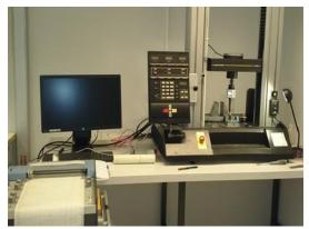
Figure (1) Universal testing machine
