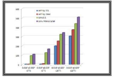
Figure 5: Static frictional force of different brackets and wires
