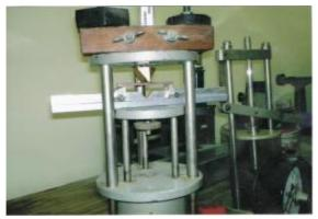
Figure 3: Flexural testing device
