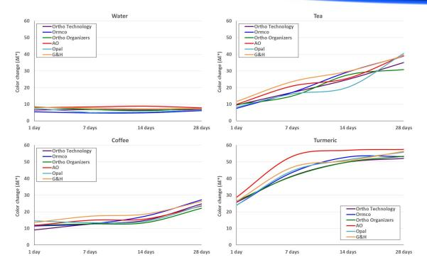
Figure 2: Color changes of elastomeric chains (Ortho Technology, Ormco, Ortho Organizer, AO, Opal and G&H) after immersion in water, tea, coffee, and turmeric.
