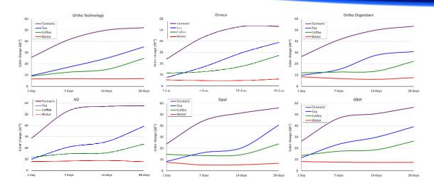
Figure 3: Mean color change of clear elastomeric chains from Ortho Technology, Ormco, Ortho Organizer, AO, Opal and G&H companies after immersion in water, tea, coffee, and turmeric.
