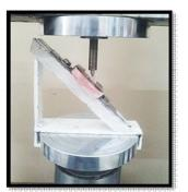
Figure 4: Die analogs mounting Figure 5: Angle of load application Figure 6: Load application in acrylic base
