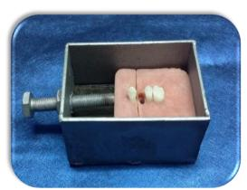
Figure 1: Template for teeth fixation.
