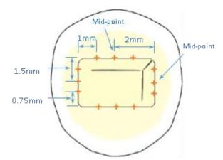
Figure 3: Points location used for the SEM examination
