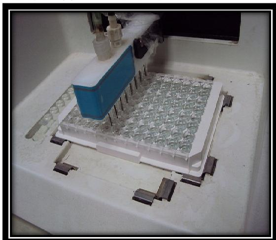
**Figure 9: Microplate ELIZA washer device**
