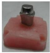
Figure 1: Finished master die with its acrylic base having seating groove at each corner
