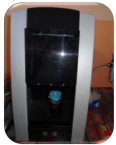
Figure 2: The scaning machine (Ceramill, Aman Girbach, Germany).
