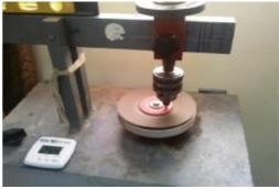
**Figure 3: Wear rate testing machine**
