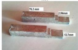
Figure 2: Mettal pattern for shear bond test
